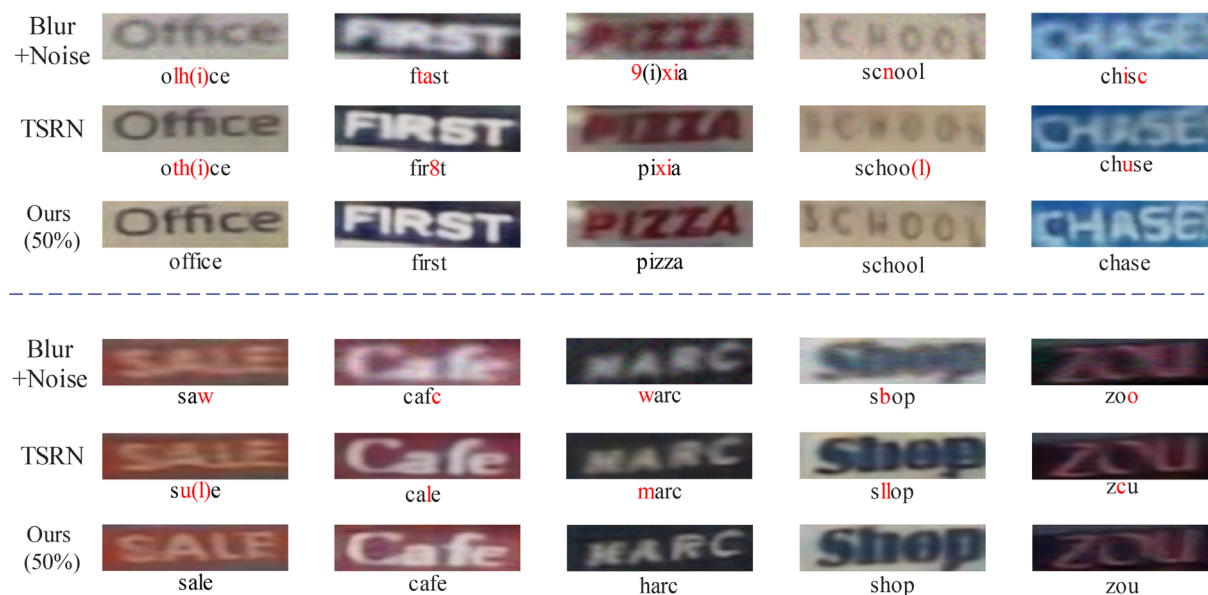
FIGURE 8 Super-resolution results of blurred and noisy images on scene text recognition datasets. Characters in red are missing or wrong. TSRN, text super-resolution network.
