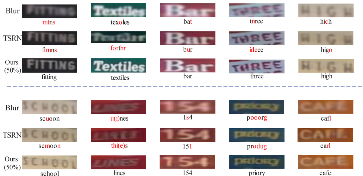
FIGURE 7 Super-resolution results of blurred images on scene text recognition datasets. Characters in red are missing or wrong. TSRN, text super-resolution network.
