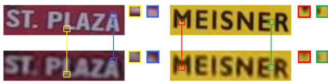
FIGURE 2 Illustration of misalignment between real-world low-resolution-high-resolution (LR-HR) pairs.
